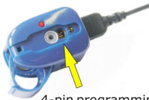
4-pin programming socket
