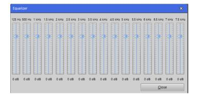
The acoustician/audiologist can adapt the hearing system accordingly to the audiogram by setting the individual frequency bands. Any potential resonance phenomena can be suppressed. This function can also linearize the frequency characteristics if required.
