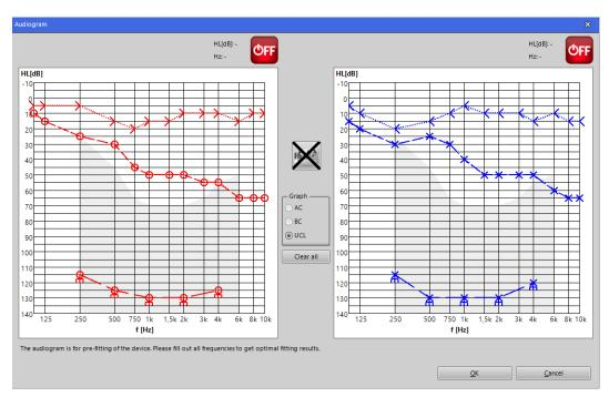
Selecting AC, BC or UCL in the **"Graph"** box enables data to be entered into the audiogram. Set data points with left-click or return key at the desired frequency (f [Hz]) and hearing loss (HL [dB]) position. The data for the <u>right</u> ear (RED) is entered in the graph on the left and the data for the <u>left</u> ear (BLUE) in the graph on the right.
